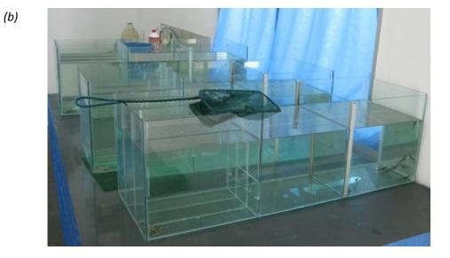
Figure 1: (a) Diagram and (b) photograph of tank used for evaluation of feeds for attractability
