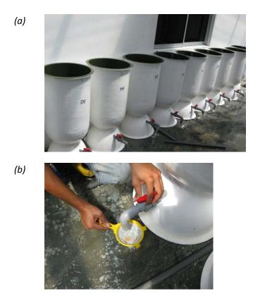
Figure 2: Photographs of tank systems used for evaluation of feeds for palatability. (a) Tank set-up; (b) Valve to collect uneaten feeds
