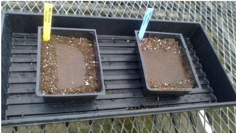
Figure 6a: MBM sheets/grass seed experiment. (Yellow- MBM/grass sandwich where each of the sandwich sheets was 0.6mm thick; Blue-MBM sheet mulch which was 0.6mm thick)
