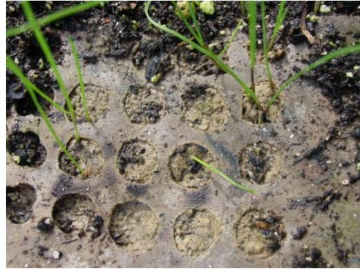
Figure 10. Multi-layer sheet (PE-MBM-grass-MBM-PE) 4"x3" of the PE sheet is perforated on either side as shown in the photo
