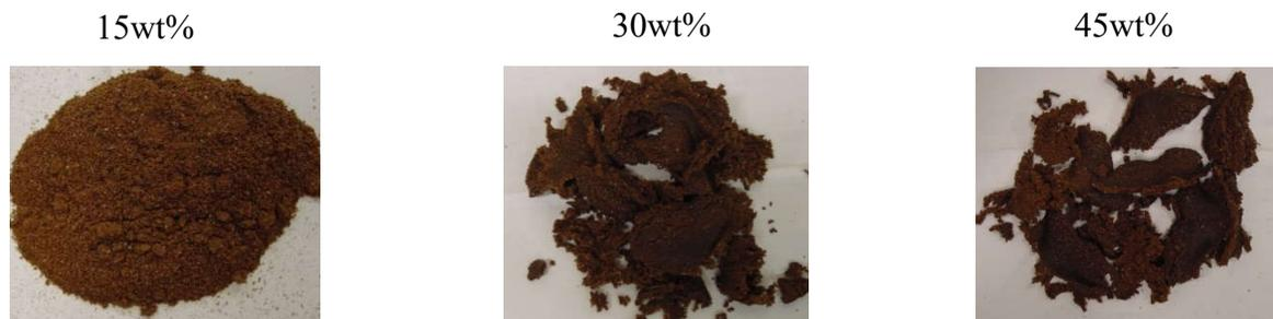
Figure 1a. Evolution of texture of compounded MBM with different plasticizer contents.
