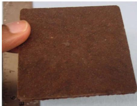
Figure 11. Thermally compacted sheet of MBM-Glycerol resin (50-50). The sheet is 3" long, 3" wide and 1.5 mm thick.
