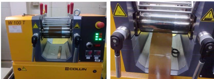
Figure 7. Calendering of MBM-LLDPE blend sheets using the Collin W 100T Calendering unit
