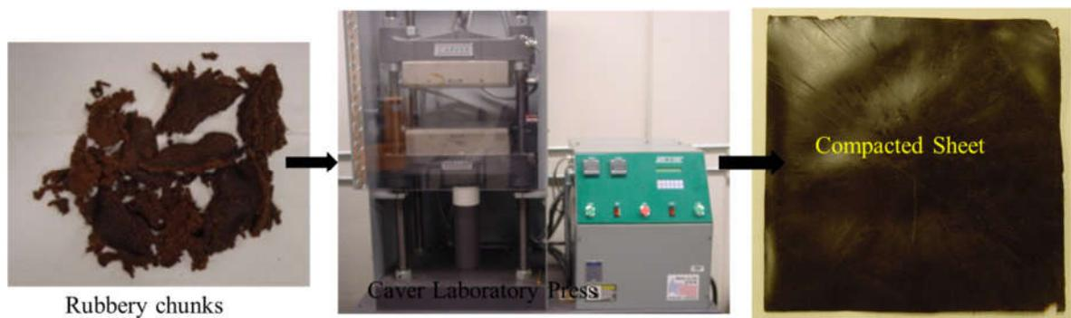
Figure 1b. Illustration of the formation of a bioplastic sheets from plasticized and batch compounded meat and bone meal.
