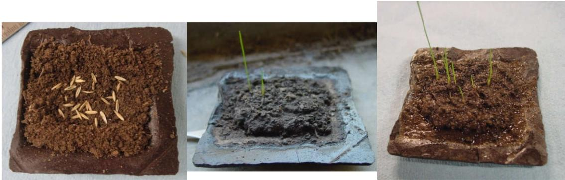
Figure 13. Investigation of seed growth support of the tray made from MBM-MAH bioplastic
