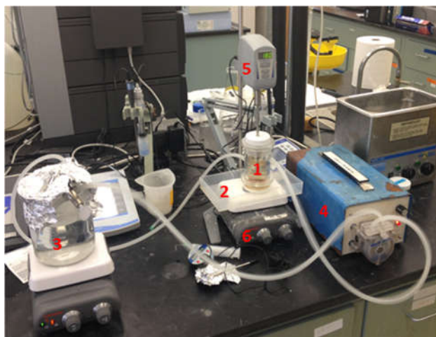
Figure 1. Forward osmosis apparatus for concentration of stick water: 1 – Concentration cell, 2 – Draw solution bath, 3 – Hot water reservoir, 4 – Peristaltic pump, 5 – Overhead stirrer, 6 – Magnetic stirrer plate.
