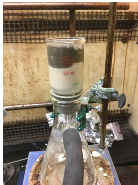
Figure 11. Experimental set-up for evaluation of clay materials for wastewater purification.
