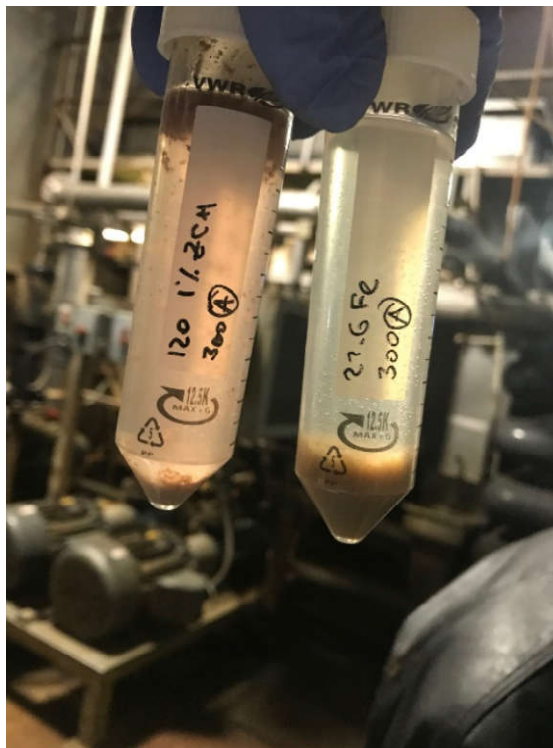
Fig. 6. Application of methylated hemoglobin in combination with currently used anionic flocculant (left) results in similar water clarification to the currently used combination of three reagents.
