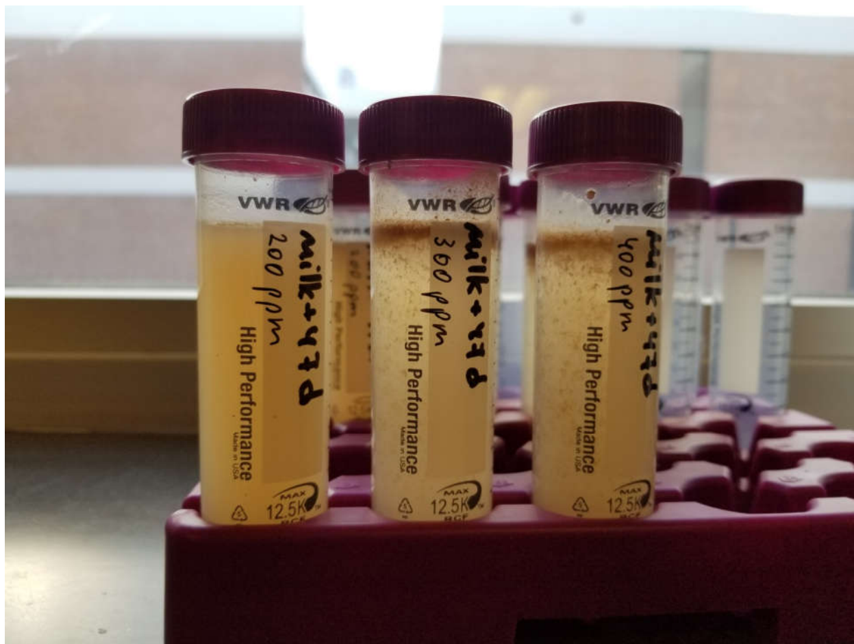
Fig.1. Effect of methylated hemoglobin on milk solution. At loading over 250 ppm clears milk solution quickly, and is very easy to filter to achieve almost clear water. 400 ppm solution after filtering was almost perfectly clear.
